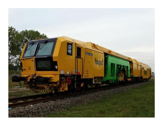
Unimat 09-4×8/4S Dynamic is a 10-axis universal tamping machine based on the operating principles of the latest Unimat 4S. The execution of track and turnout alignment works in vertical and horizontal planes with simultaneous stabilization of the track structure is combined in one universal machine.
